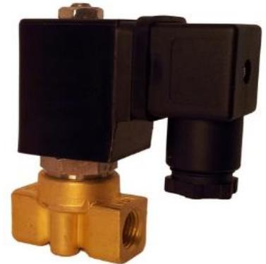
The ST-DA is a direct operated 2/2-way solenoid valve. The valve is normally closed. The solenoid valves have an orifice of 3 mm, operate from 0 bar and are suitable for small flow rates. The body material can be brass, nylon or stainless steel with a NBR, EPDM or FKM seal. The ST-DA solenoid valves are compatible with all coils from the CS1-series.
